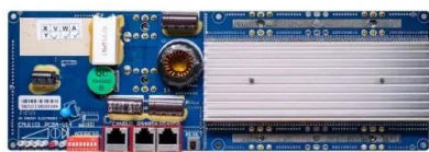
ES485 Communication between battery and inverter Bit rate: 9600bps ES485 Interface Communication between power packs or BMS and PC Bit rate: 9600bps
